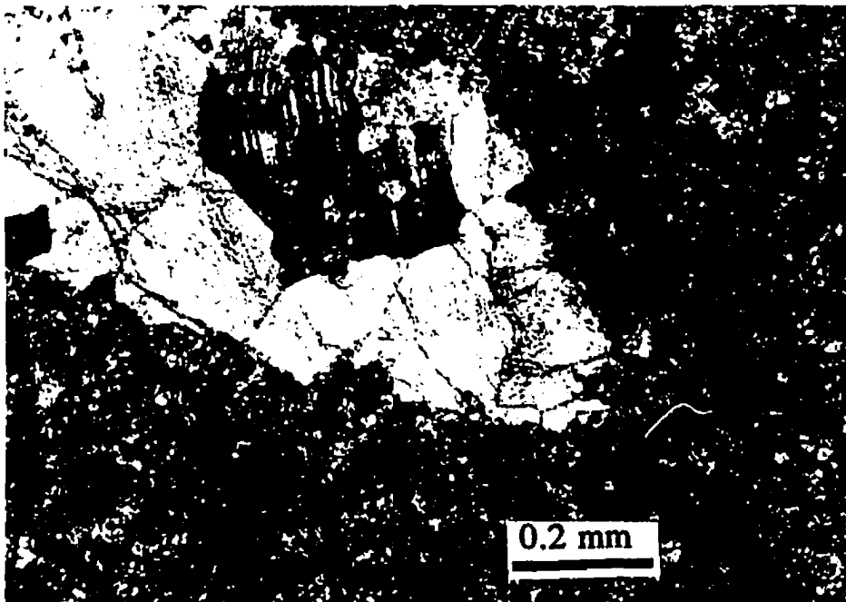
Plate 3.2. Vein calcite cement is crosscut by stylolites (filled by black bitumen).
